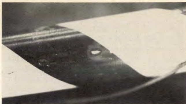
FIG. 7 Pit marks where flash attached
