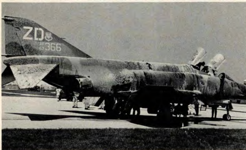
Jettison of three external tanks to reduce landing weight also got rid of the source of the fire. The crew brought this one back after an adrenaline-filled eight minutes. Photo on right shows centerline bomb rack from below.
