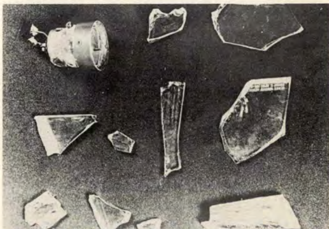
FIG. 10 NAV light globe broken by lightning, leaving a path for lightning current to enter aircraft's electric system.
